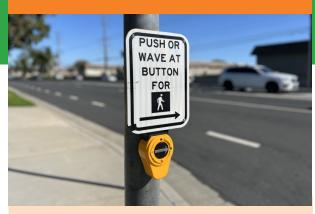
In an ongoing effort to enhance pedestrian safety and accessibility throughout Cypress, we are installing accessible pedestrian signals (APS) citywide. APS devices are equipped with audible and vibrotactile features, ensuring inclusivity for all community members.
